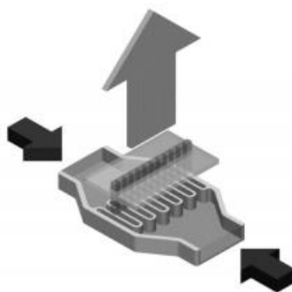
Fig 1. Representation of the multi-lamination principle. Interdigital flow passes slit to create multi-lamellae.
